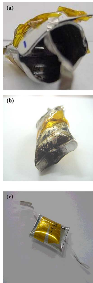
Fig. 4. Pictures of cell external appearance after 2C overcharging experiments.
